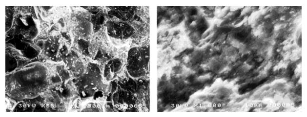
**Figure 12** SEM micrograph of polyester mortar composite before being immersed in sulphuric acid solution.
