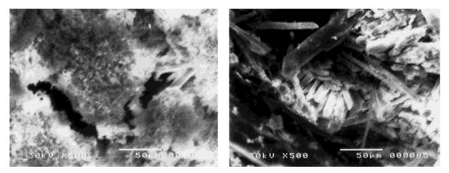
**Figure 11** SEM micrograph of hardened cement mortar after being immersed in 10% sulphuric acid solution for 60 days.
