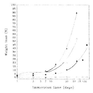
**Figure 1** Weight loss of cement mortar as a function of immersion time in: ( $\Box$ ) distilled water, ( $\blacksquare$ ) 5%, ( $\triangle$ ) 10%, and ( $\blacktriangle$ ) 15% H<sub>2</sub>SO<sub>4</sub> solutions.
