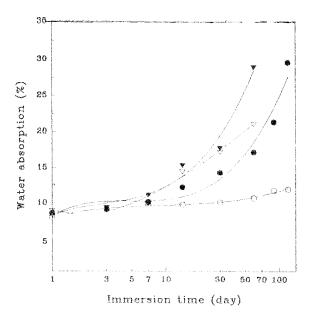
**Figure 7** Water absorption of cement mortar as a function of immersion time in: ( $\bigcirc$ ) distilled water, ( $\bigcirc$ ) 5%, ( $\bigtriangledown$ ) 10%, and ( $\bigtriangledown$ ) 15% H<sub>2</sub>SO<sub>4</sub> solutions.
