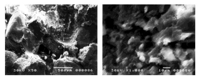
**Figure 13** SEM micrograph of polyester mortar composite after being immersed in 10% sulphuric acid solution for 60 days.
