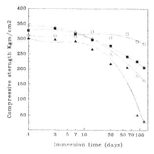
**Figure 4** Compressive strength of polyester-impregnated cement mortar as a function as a function of immersion time in: ( $\Box$ ) distilled water, ( $\blacksquare$ ) 5%, ( $\triangle$ ) 10%, and ( $\blacktriangle$ ) 15% H<sub>2</sub>SO<sub>4</sub> solutions.
