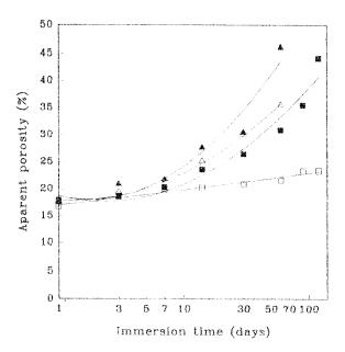
**Figure 5** Apparent porosity of cement mortar as a function of immersion time in: ( $\Box$ ) distilled water, ( $\blacksquare$ ) 5%, ( $\triangle$ ) 10%, and ( $\blacktriangle$ ) 15% H<sub>2</sub>SO<sub>4</sub> solutions.
