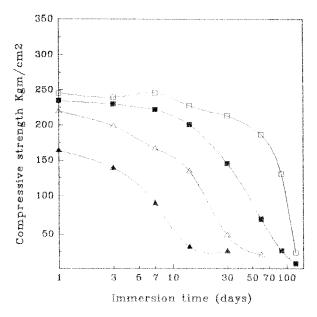
**Figure 3** Compressive strength of cement mortar as a function of immersion time in: ( $\Box$ ) distilled water, ( $\blacksquare$ ) 5%, ( $\triangle$ ) 10%, and ( $\blacktriangle$ ) 15% H<sub>2</sub>SO<sub>4</sub> solutions.
