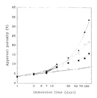
**Figure 6** Apparent porosity of radiation-treated polyester-impregnated cement mortar as a function of immersion time in: ( $\Box$ ) distilled water, ( $\blacksquare$ ) 5%, ( $\triangle$ ) 10%, and ( $\blacktriangle$ ) 15% H<sub>2</sub>SO<sub>4</sub> solutions.
