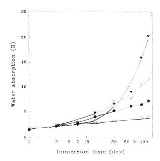
**Figure 8** Water absorption of polyester-impregnated cement mortar as a function of immersion time in: ( $\bigcirc$ ) distilled water, ( $\bullet$ ) 5%, ( $\bigtriangledown$ ) 10%, and ( $\checkmark$ ) 15% H<sub>2</sub>SO<sub>4</sub> solutions.
