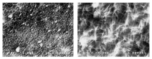
**Figure 10** SEM micrograph of hardened mortar before being immersed in sulphuric acid solution.
